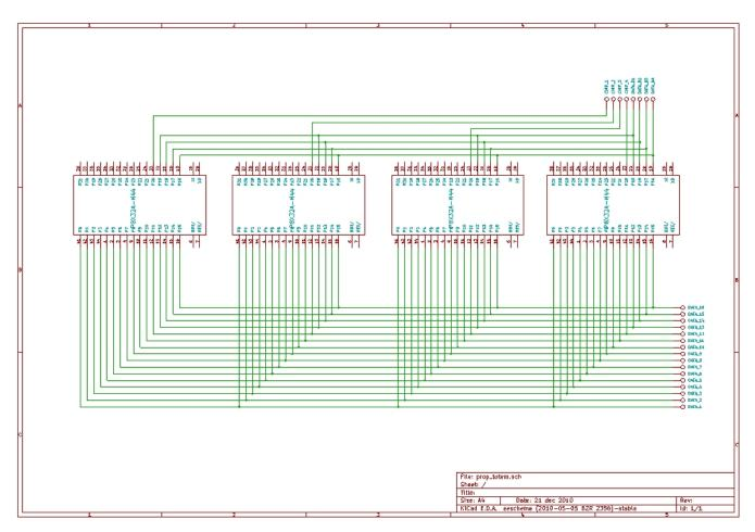
Totem stacking setup (EEPROM (or FRAM) and MEMS/crystal oscillators omitted):
