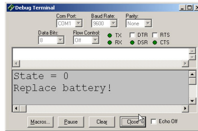
Figure 2-40: Debug Terminal Good and Low Battery Tests
