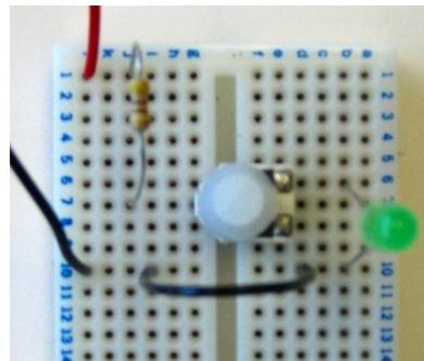
Now, when you plug the battery into the clip, the LED should become brighter or dimmer depending on the direction of rotation.
