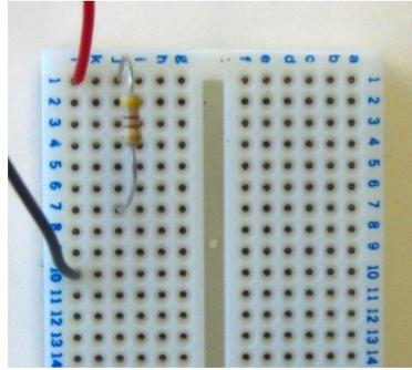
Now it's time to connect the potentiometer. According to the schematic, the wiper pin of the potentiometer is connected to the other end of the resistor.
