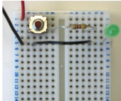
And you've successfully wired your second circuit! Just connect your battery and verify that when you press the button, the LED lights up.
