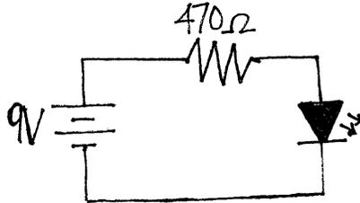
By looking at the schematic we can identify a few symbols from our list: a battery supplying 9V, one  $470\Omega$  resistor, and one LED. In order to wire this on a breadboard, it's easiest if you just take each component one at a time.
