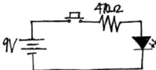
The pushbutton is interesting in that it has four pins, but is only represented in a schematic by two. This is because the pushbutton needs all four pins for stability, but only two for functionality. The two pins not shown in the schematic symbol are electrically connected to the two pins that are shown and therefore not necessary to picture.
