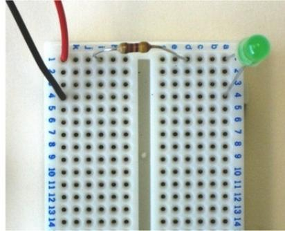
Finally, the cathode of the LED is connected to the negative terminal of the battery, like so:
