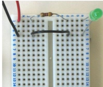
And congratulations, you've successfully wired a circuit from a schematic! That wasn't so horrible, was it? Now if you plug a battery into the clip, the LED should light up.
