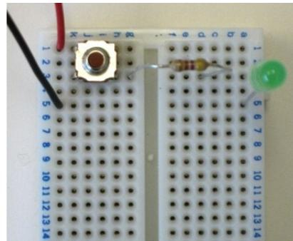
And finally, the cathode of the LED is connected to the negative terminal of the battery:
