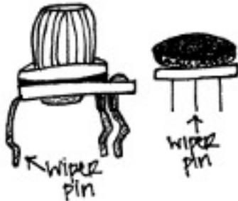
Potentiometers come in all sorts of shapes and sizes, but their functionality remains the same across most types. They have three pins, two of which make up the total resistor value, and a third called the wiper. The wiper is the actual mechanism that changes the resistance value as you rotate the dial. This is normally the center pin on most potentiometers, and an example drawing of two commonly found potentiometers can be seen to the left.
