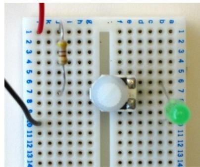
Lastly, the LED's cathode is connected to the negative terminal of the battery to complete the circuit.
