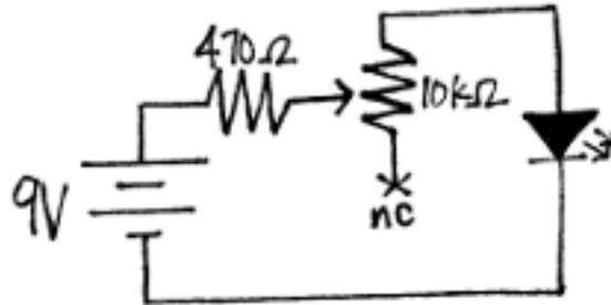
The potentiometer is also known as a variable resistor which, as its name implies, has a resistance that changes. The 10kΩ marking next to the schematic symbol indicates the maximum resistance value the potentiometer has.
