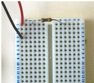
Then, the other end of the resistor is connected to the anode (or long lead) of the LED:
