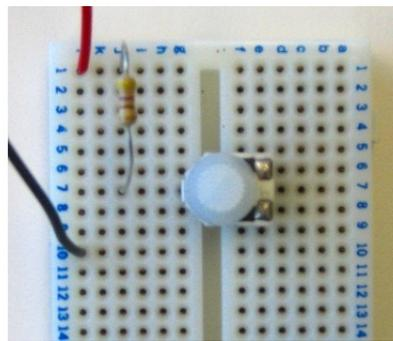
The LED's anode is then connected to the top pin of the potentiometer, like so:
