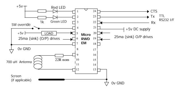
The H4001 based transponders provide 64 bits of read-only memory. This memory contains a header bit sequence and 40 bits (5 bytes) of user data interspersed with parity bits. Data is only accepted from the H4001 transponder if the memory parity bits are valid. This configuration ensures that the integrity of user data is maintained. The H4001 transponder type is widely used throughout the world in its base form and also in many fully compatible derivative forms.
