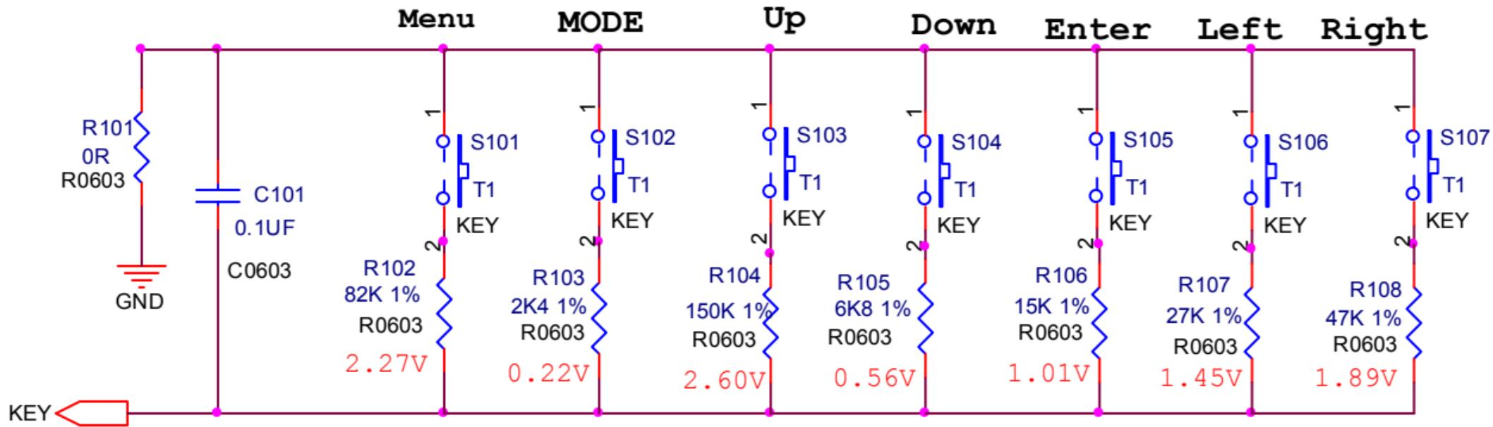
Note: the keyboard input of DSP is connected to internal ADC circuit, thus, the accuracy of the resistor is important in this application
