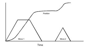
The ramp function used in the Little Step-U is a piecewise, linear ramp of frequency in 64 steps. The motor is run at each of these speeds for a period that is 1/64 of the ramp time requested with the {B} command.
