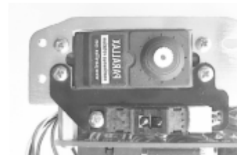
Figure 1.9: IR wheel encoder detectors mounted on chassis.
