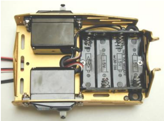
Figure 1.11: (a) Battery pack installed
