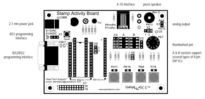
I/O pins brought out to standard 2x10 IDC header for easy access. Four pushbuttons and LEDs for operator interface. (Actual size = 4.00" x 3.00")
