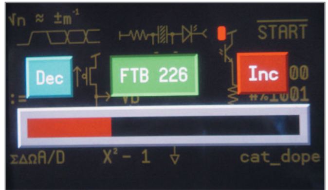
Photo 3 —This photo of my VGA monitor's screen shows the simple display of three buttons with a horizontal gauge on a background of random characters and graphics. The red spot is the mouse cursor used to select a button. The buttons change a variable whose value determines the gauge's length. This data could come from an internal cog running a sampling application or from an external processor using the Propeller strictly as a display device.
