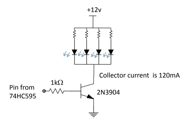
This configuration would be on each of 20 output pins.
