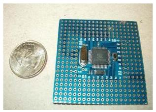
Hippy <u>suggested</u> a retangular cut, allowing pins to be brought out on either side for breadboard use, my own square cut left room for placement of video/audio resistors as well as connections for an SD interface. A minimal connection might just use the single row of connection holes closest to the chip itelf. Keep in mind this is one of those measure twice, cut once situations.
