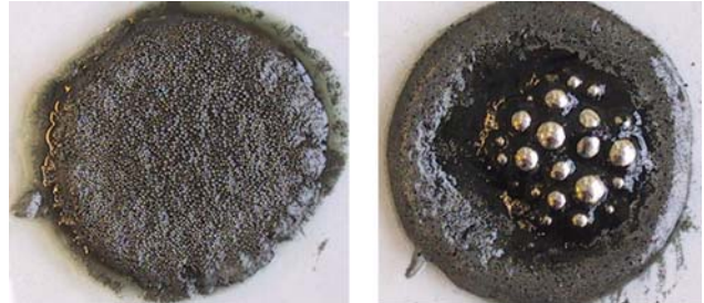
Figure 4. Preliminary test for microwave soldering with a BiSn solder paste with (right) and without (left) suszeptor additions
