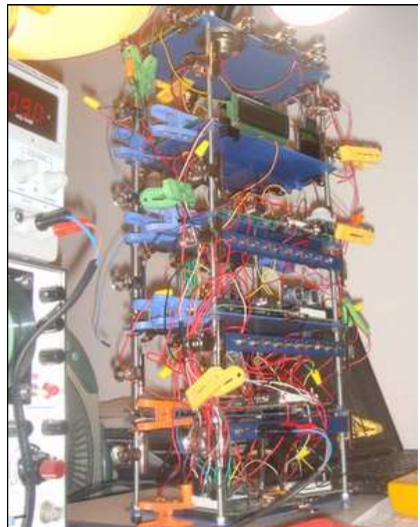
The Basic Stamp Supercomputer contains a growing cluster of 11 Basic Stamp processors, & peripherals.
