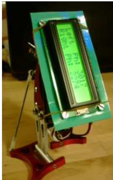
Penguin works with Parallax LCD models 27977 and 27979, using Vittorio Rossi's Penguin LCD Monitor code. The LCD is simply held in place with elastic bands.
