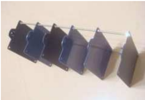
Left- a rack is made from half size clipboards found at a dollar store. Threaded rods came from Home Depot. Right- computer 9 has EMIC TTS text to speech running in ascii mode. The interface was simplified to three wires with handshaking. The external speaker is mounted under the top rack level. What about EMI, RFI interference? The lateral surrounding ground wires provide shielding.
