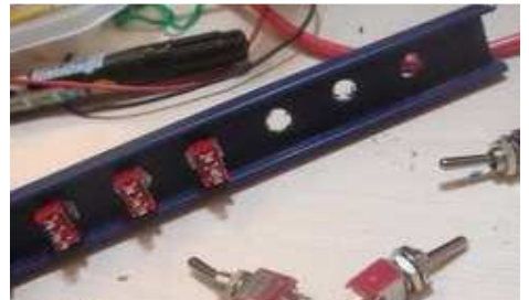
Left- photo shows the Master being built and talking to the LCD. This is the first LCD test using a Parallax/ Scott Edwards BPI-216 serial LCD. Later versions have the yellow LED replaced with red. Right- a plastic hanger base is machined to fit switches. A Taiwan hobby tool (lower right) was used to drill holes, cut lengths and remove burrs.
