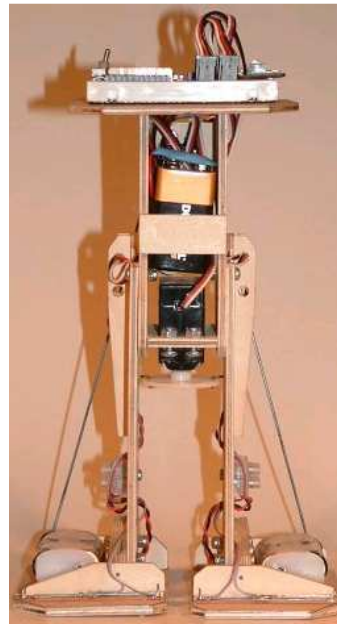
With his famous two-servo design, David Buckley built Pop and Mom, 2-legged walkers made from wood.
