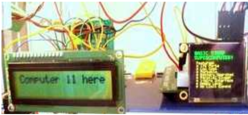
Left- LCD monitor shows computer (Basic Stamp) number 11 talking to the Master. The LCD monitors all Super computing traffic on the "Supernet." Right- boards easily pull off the rack for testing, wiring and modifications.
