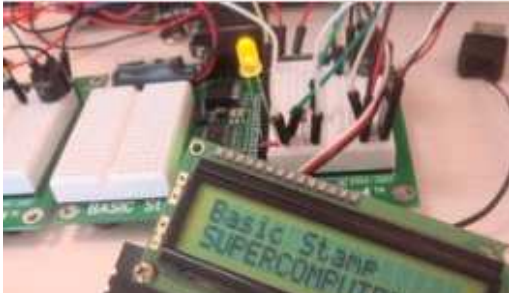
Left- photo shows the Master being built and talking to the LCD. This is the first LCD test using a Parallax/ Scott Edwards BPI-216 serial LCD. Later versions have the yellow LED replaced with red. Right- a plastic hanger base is machined to fit switches. A Taiwan hobby tool (lower right) was used to drill holes, cut lengths and remove burrs.
