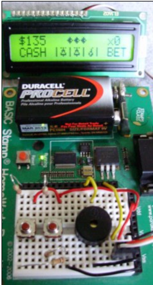
Above- Photo shows the Basic Stamp II LCD Slot Game created using a HomeWork Board. Below-LCD display shows the current bet, cash and spin indicator – realism on a simple two line LCD. Photos & schematic by Mike Donahue.
