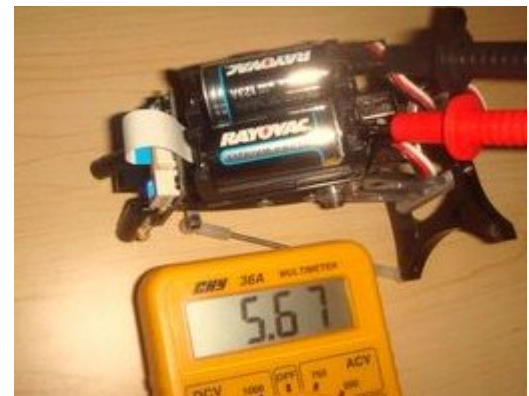
Left - use several built-up layers of tape as a short term light shield. Right - to measure voltage, connect positive (red +) and negative (black -) leads to the two metal tabs on the bottom of the CR123A holder. The measurement shown is the combined voltage of two batteries in series.
