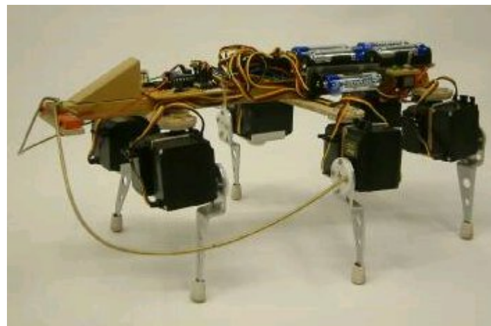
David Buckley built Simplhex, a six legged walker with a wooden chassis and aluminum legs. A newer Simplex clone uses all wood.
