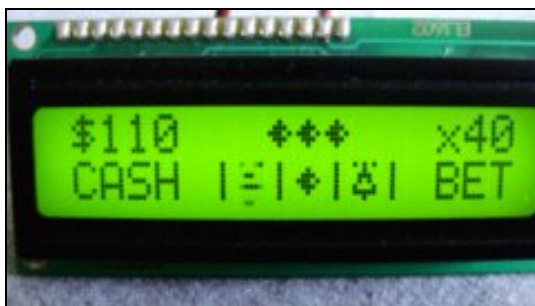
Above- Photo shows the Basic Stamp II LCD Slot Game created using a HomeWork Board. Below-LCD display shows the current bet, cash and spin indicator – realism on a simple two line LCD. Photos & schematic by Mike Donahue.
