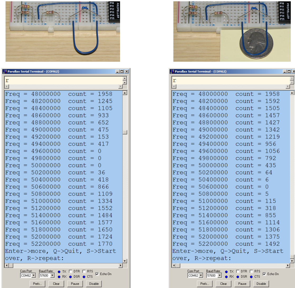
Figure 31: Calibrated Metal Detector Response – without metal (left) and with metal (right)
