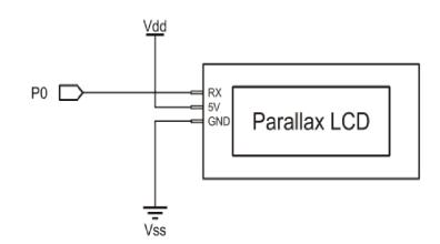
An LCD module is a "must have" for any Propeller experimenter. The Parallax serial LCD (part#27979) displays four lines of data with a backlight for easy viewing. You'll also want a Parallax LCD Extension cable (part#805-00012) as the LCD module doesn't plug directly into a beadboard well. The extension cable is packaged with a male-to-male three pin header allowing easy an easy connection between the the breadboard and the cable.
