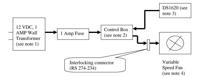
Note 1: The wall transformer may be a switching or regular transformer type. The switching type is smaller and lighter than the transformer type; however, the transformer type will probably have better life expectancy. Switching transformer - SCEPTRE POWER, Model# AMDD-20120-1000, P/N: PX1210AWPL05, INPUT: 100-240 VAC 50/60 Hz 0.5 A, OUTPUT: 12.0 VDC 1 A.
