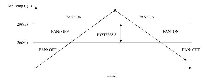
Fan is ON When DS1620's Tcom Pin is HIGH And IRL520 Is Conducting.Fan is OFF When DS1620's Tcom Pin is LOW And IRL520 Is NOT Conducting.
