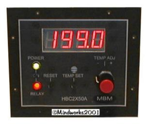
Once the Set Temperature of 708F has been reached, the Red Relay Led turns off and the internal buzzer sounds off three times indicating that the Set Temperature has been reached....
