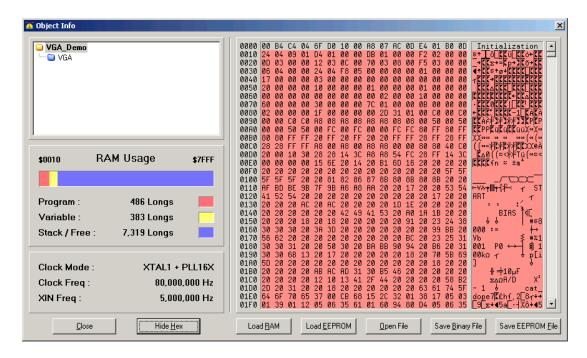
5. Select 'Save EEPROM File' and navigate to where you put the GEAR executable files and hit the save button, modify the file name if you want, then complete the save.
