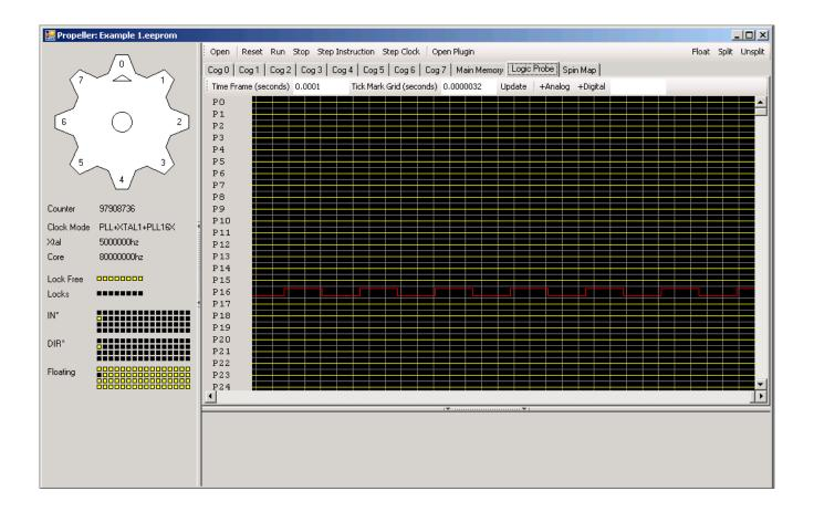
As shown pin 16 is colored red, for output. At the left, you can also see the pin state registers and the state of pin 16 there too.
