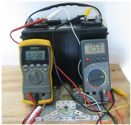
polarity. Theoretically the motor armature should continue to accelerate to a higher and higher speed unless there is a force that works in opposition to the battery voltage. Clearly the motor armature does not continue to accelerate but instead reaches a finite top speed.
