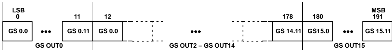
Figure 8. Grayscale Data Packet Format
