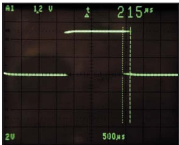
Photo 2 —The TSL230R's frequency output displayed on my oscilloscope shows a slow frequency jitter marked by the vertical cursors. The output frequency shifts with the varying amount of light absorption because of the blood pulsing within the light's path.
