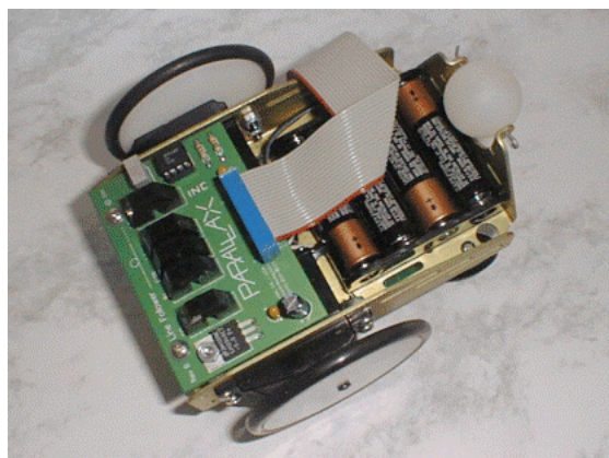
Figure 1: The Mounted Line Follower Module
