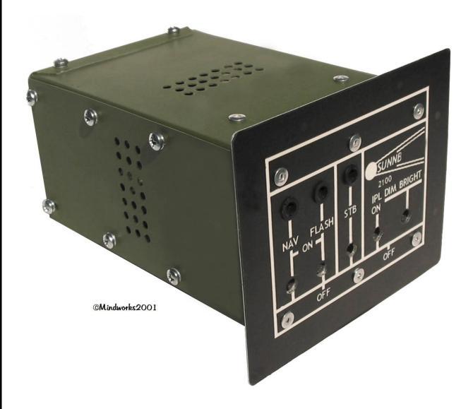
Picture NSI 4....Here is another example of an Enclosure with the electronic components removed for final color coating. This enclosure is primed with green zinc chromate for corrosion resistance. The measurements are 3-1/2" W x 5-11/16" D x 2-3/4" H ....
