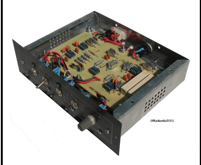
Picture NSI 2....Here is an internal view of the NSI 1 showing the two custom made PCB's. One on top of the other. Very Compact....
