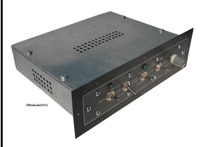
Picture NSI 1....This Enclosure, Label and Electronics was designed for an Experimental Aircraft which controls the Navigation, Strobe and Instrument panel Lights....This Panel mounted Enclosure is approximately 7-3/8" W x 6" D x 1-1/2" H ....
