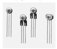
Disc-type EMIFIL® DS310, DST310 and DSS310 are T-type EMI suppression filters. The disc-type EMIFIL increases the self-resonant frequency of the capacitor by attaching two lead wires to one of the electrodes of the capacitor and increases the insertion loss by adding inductance to the lead in the DST and DSS types only. Frequencies to be suppressed can be selected by choosing the capacitance. They are also recommended for use as by-pass capacitors.
