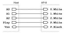
When using parallel input control the segment select dip switches 0..2 must be left in the Open position.
