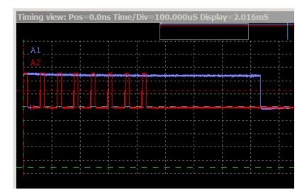
Below is the timeout after initialization (Blue line). It has been shortened to the data rate of 8 bits. This allows any errors in sending data to be processed faster than an arbitrary timeout. Error flags for timeout conditions can be read with the ERROR command.
