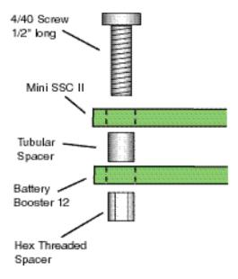
The 1/4" long 4-40 thread screws are used to attach the Mini SSC II / Battery Booster 12 assembly to a baseplate on your robot or animatronic. Here are the dimensions of the Battery Booster 12/Mini SSC II mounting holes:
