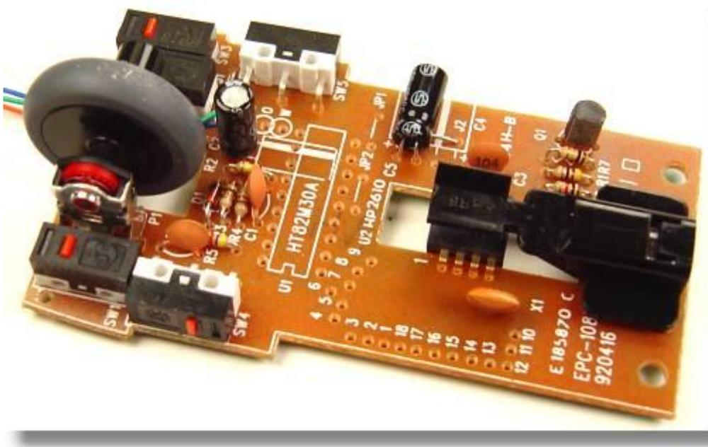
Remove the orange and white wires connected to the mouse cable and reconnect them to the pins 6 and 7 shown here. These are the IO clock and data ports to the 2610 chip.
