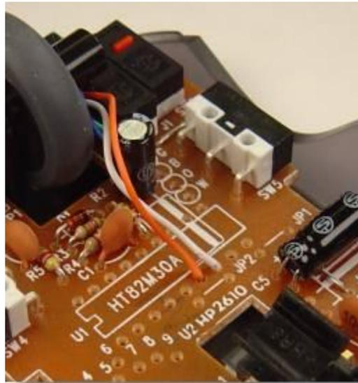
Cut the end of the cable and connect the wires to a small 4 pin header as shown. The color codes are as follows:
