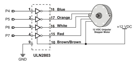
From a microcontroller's standpoint, causing the motor to take a "step" involves taking two pins "high" at a time through the driver circuit shown above.
