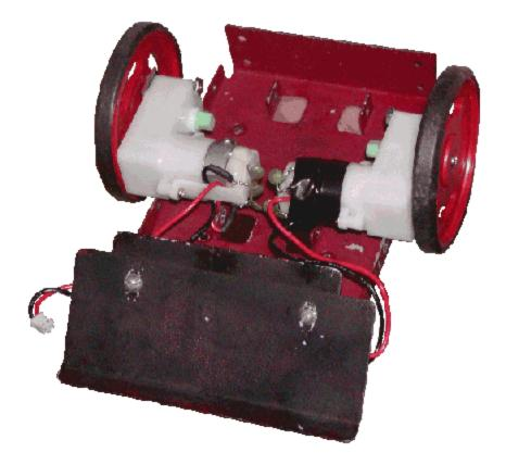
We had to drill new holes exactly 1/2" farther forward than the two back holes for the standoffs on the chassis. This was necessary to allow the gearmotors to fit in between the mainboard's standoffs.
