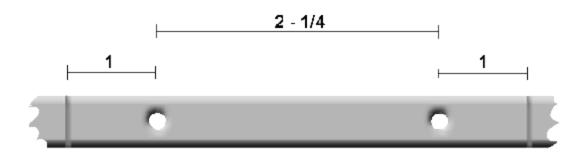
We scribed all the measurements onto the aluminum by covering most of one side of the piece of aluminum with permenant marker. Then we scribed the lines on with a combination square.
