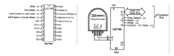
3) Connect the encoder to the encoder interface chip. Use the power supply and ground from the BSII to power the encoder.
