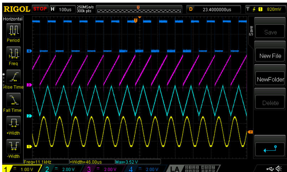
Fig. 17 A scope trace acquired while the P2 is running in 4 channel DDS mode, this time outputting waveforms pre-calculated in the P2's LUT.
