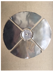
Figs. 18a and 18b Home brew electrode set for Goertzel quad experiments (left) and data trace as my hand/finger are moved above and around the electrodes (right).
