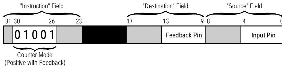
Figure 3: CTR x Register Configured for Sigma-delta Operation
