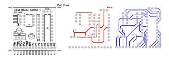
The above images of the board layers are not to scale. Please visit <a href="www.parallaxinc.com">www.parallaxinc.com</a> for the actual source and gerber files. This board was designed using Protel's Client '98 software. The top copper layer is the center plot, and the bottom copper layer is as 'viewed through' the board. Here's the schematic:
