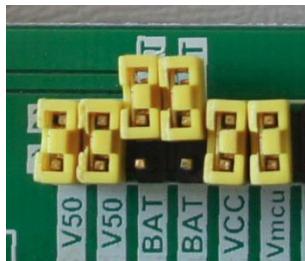
Battery jumpers in OFF position
