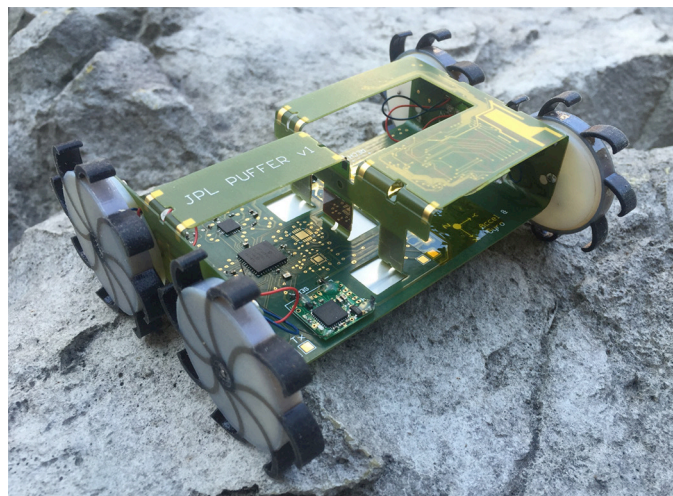
PUFFER prototype incorporating a folding printed circuit board as its pop-up structure.
