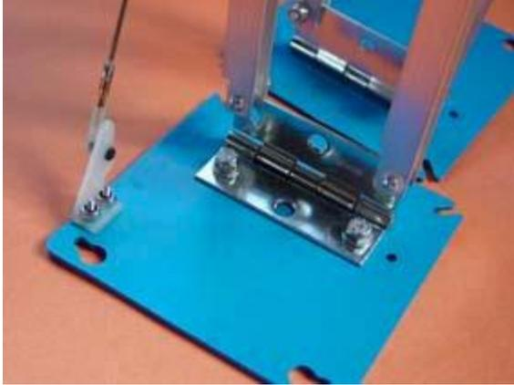
Here is a detail of the foot. It is made from a 4"x4" plastic outlet box cover and a hinge. 3/4" felt pads are on the bottom to protect hardwood floors etc.
