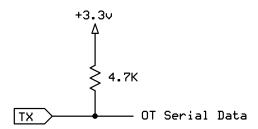
For *Open-Inverted* mode the Propeller will drive the line high for a start and zero bit, and let it float for a one bit and stop bit. Since the polarity is inverted we need to add a pull-down resister to the serial pin.
