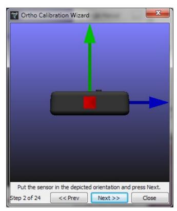
Put the sensor in that orientation and press Next, making sure to hold the sensor still until the picture moves
