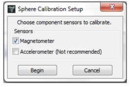
When performing calibration, a large sphere will appear that represents possible magnetometer and accelerometer vectors that will be collected as the sensor is rotated.
