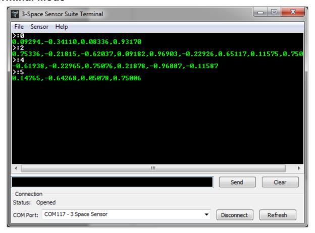
Terminal mode allows you to communicate directly with the sensor without the aid of the graphical interface. For instructions on how to communicate using terminal commands, see the 3-Space Protocol Reference document.
