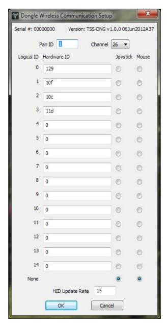
On this screen, enter the serial number of a wireless sensor into the address slot you would like to communicate with it on. You may later select that address in the Sensor Select box on the main window to communicate with that sensor.
