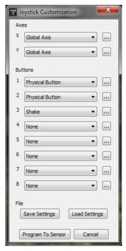
The joystick and mouse on the sensor are represented as a series of configurable virtual axes and buttons. This window allows you to change the way the axes and buttons on either the joystick or mouse function. Each axis and button has a number of operation modes you can choose from.
