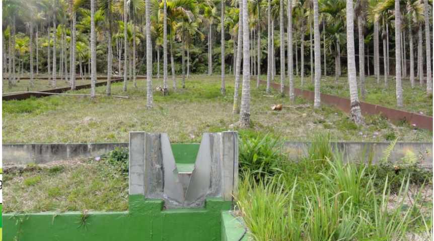
The example of USLE standard size plot (Taiwan) consisting of triangular weir, a water level sensor, the reservoir of earth and sand.
