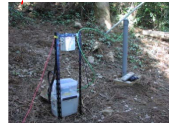
Groundwater sampling using the pump (the right) in observation well (water level monitoring) (the left)
