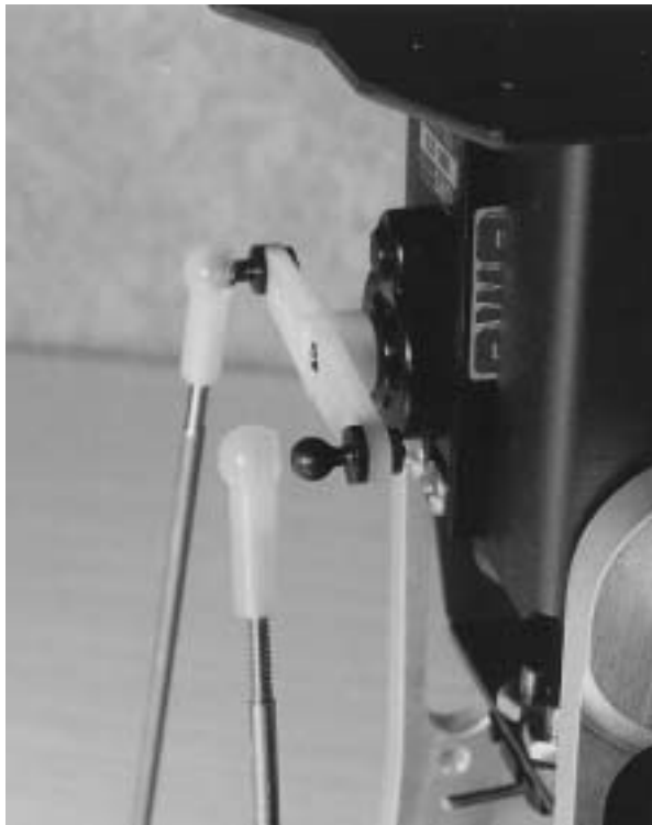
Figure 1-17 Install tilt rods
