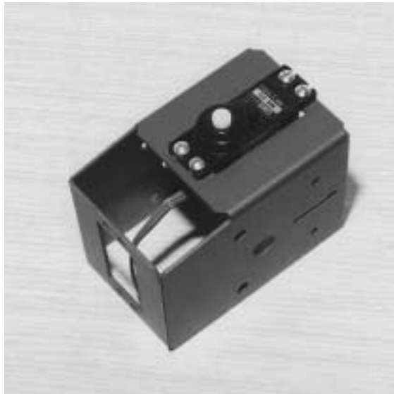
Figure 1-1 Install Tilt servo in body
