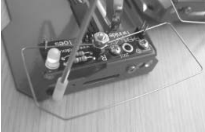
Figure 8-5: Twinkle Toes include the pushbutton resistors and bi-color LED.
