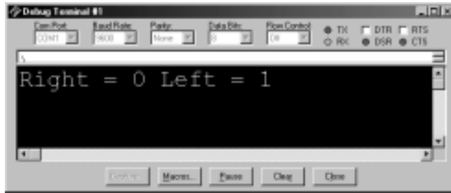
Figure 8-6: Toddler Toes DEBUG Test. Pushing the bumper should result in a “0” on the I/O pin.
