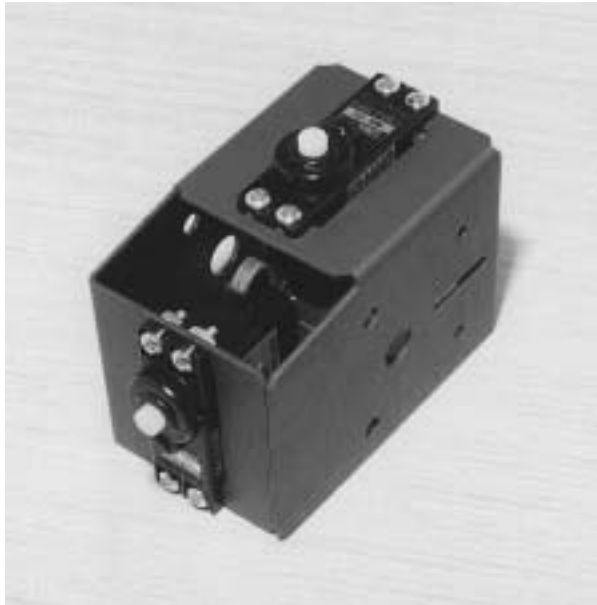
Figure 1-2 Install Stride servo in body
