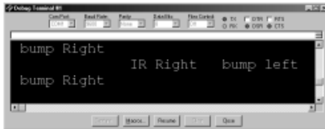
Figure 8-7: Toddler Toes and Infrared DEBUG Test. The sensors that detect an object will be shown in the DEBUG window.
