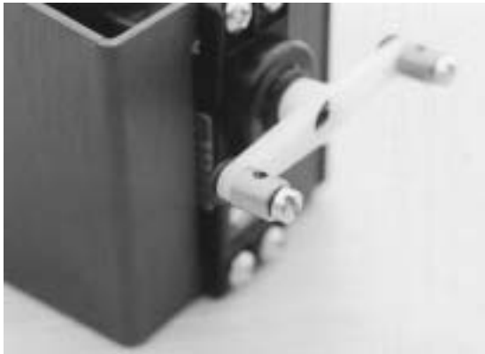
Figure 1-6 Put the two set screws back into the brass wire keeper so they don't get lost.
