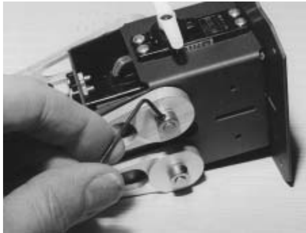
Figure 1-10 Use the 3/16" metal collars. Be sure legs move fairly freely against the body.
