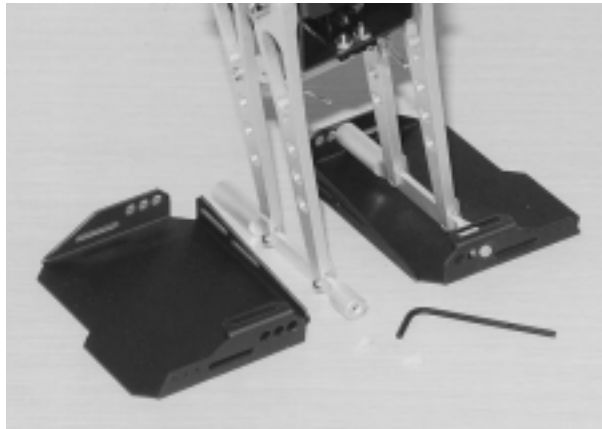
Figure 1-14 Attach feet with alan-cap screws
