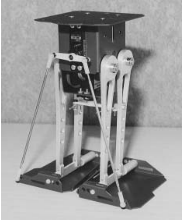
Figure 1-18 Final installation of tilt rods
