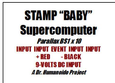
Fig. 5 The front Banner is a label denoting various functions, such as switch and plug function. It shows five switches, including a toggle for an event in time, software reset or condition notification, four input toggle switches (for data, flags, configurations, stats, debugging), and two 9-volt DC power inputs with positive (red) and negative (black) polarity.
