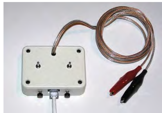
Figure 3.5-3: A Completed Control Box
