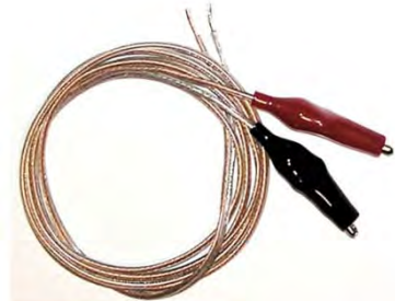
Figure 3.2-3: Completed Power Cord
