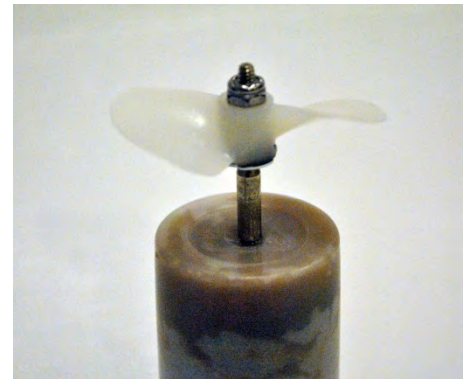
Figure 2.6-2: Propeller and Shaft Coupler Mounted on a Thruster Motor's Shaft
