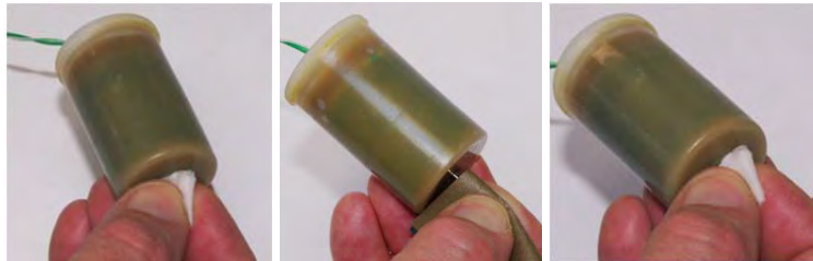
Figure 2.5-1: Cleaning, Roughening, and Re-cleaning a Motor Shaft
