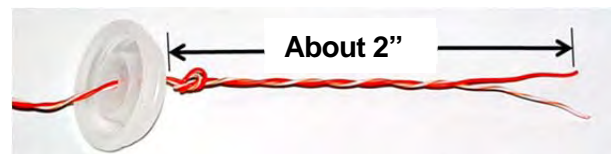
Figure 2.3-5: A Motor's Wires Passed through a Thruster Housing Cap and Knotted
