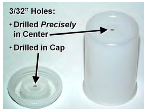
Figure 2.2-1: Holes Drilled in Thruster Housings
