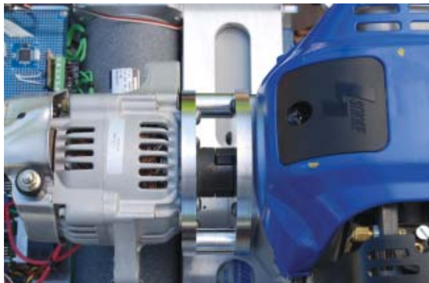
A direct coupling between the engine and alternator requires minimal space and looks really clean. This approach is also safer, since there are no belts to catch your fingers.
