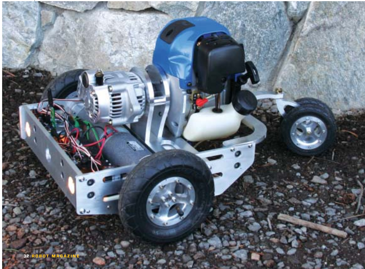
Electronics are in the front of the robot (that's a Propeller Proto Board on the left). The Ping))) ultrasonic distance sensors are built into six locations around the perimeter of the chassis.
