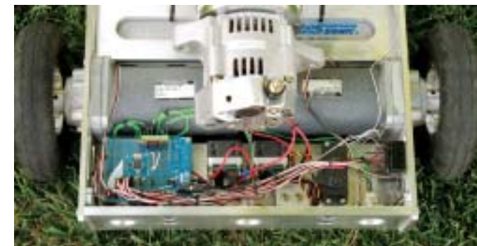
Electronics are in the front of the robot (that's a Propeller Proto Board on the left). The Ping))) ultrasonic distance sensors are built into six locations around the perimeter of the chassis.
