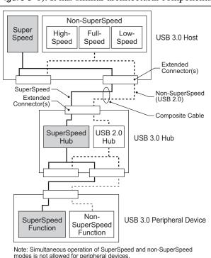
Figure 3-1. USB 3.0 Dual Bus Architecture
