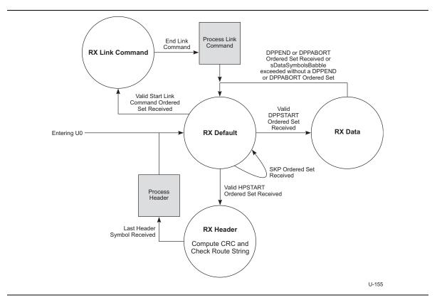
Figure 10-17. Upstream Facing Port Rx State Machine
