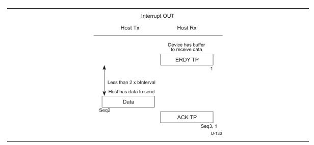
Figure 8-42. Host Resumes Sending Interrupt OUT Transaction After Device Sent ERDY
