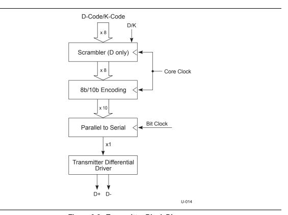
Figure 6-2. Transmitter Block Diagram
