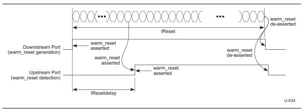
Figure 6-22. Example of Warm Reset Out of U3
