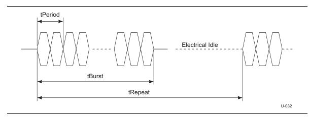
Figure 6-20. LFPS Signaling
