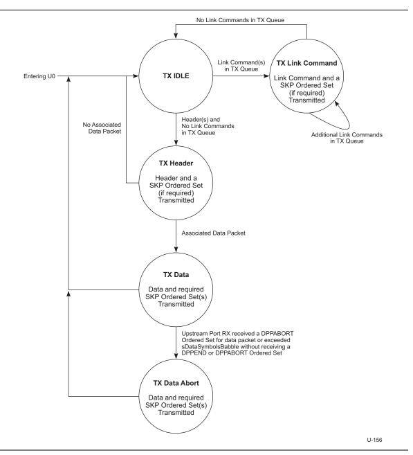
Figure 10-18. Downstream Facing Port Tx State Machine
