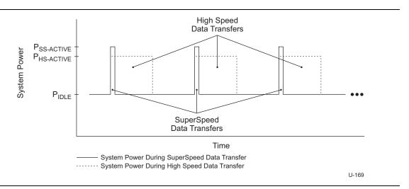
Figure C-9. System Power during SuperSpeed and High Speed Device Data Transfers
