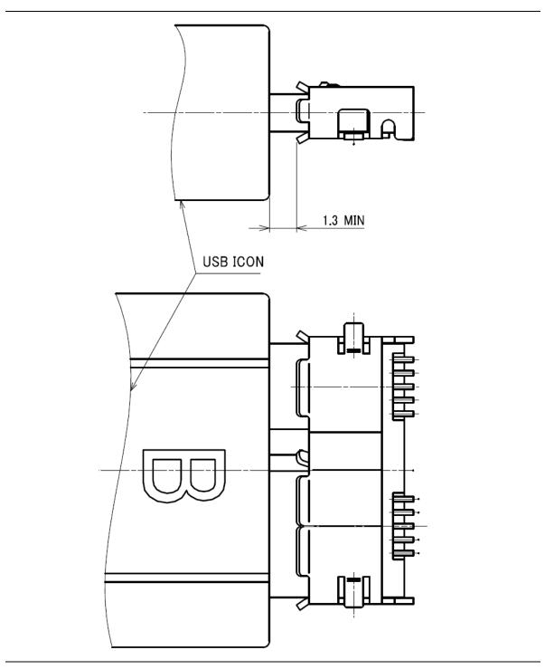
Figure 5-30. Mated USB 3.0 Micro-B Connector
