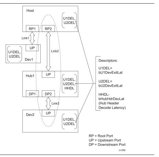
Figure C-5. Device Connected Through a Hub
