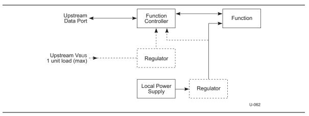
Figure 11-4. Self-powered Function
