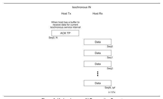
Figure 8-46. Isochronous IN Transaction Format
