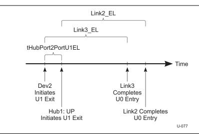
Figure C-7. Upstream Device to Host Path Exit Latency with Hub
