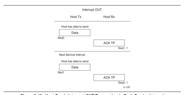
Figure 8-40. Host Sends Interrupt OUT Transaction in Each Service Interval
