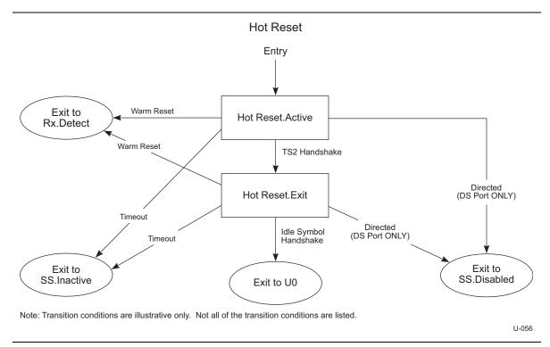
Figure 7-22. Hot Reset Substate Machine
