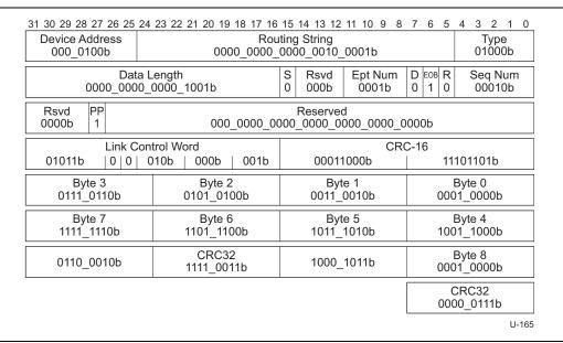
Figure D-2. Sample Data Packet
