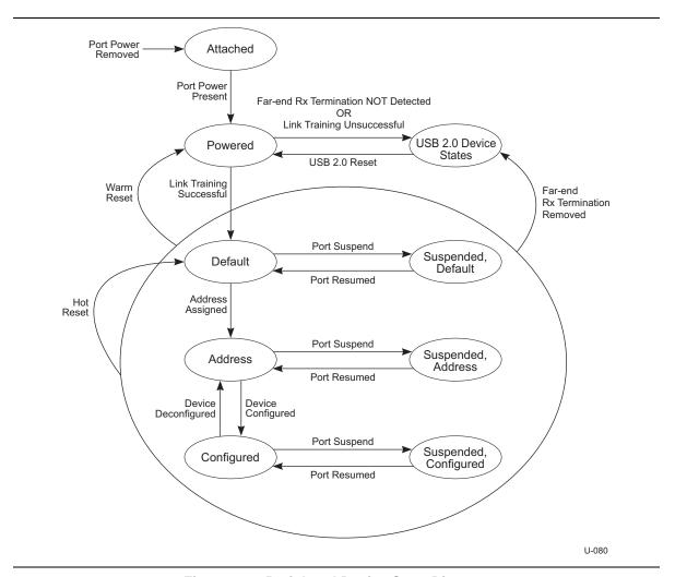
Figure 9-1. Peripheral Device State Diagram
