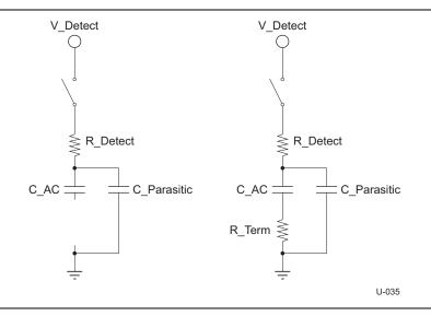
Figure 6-23. Rx Detect Schematic
