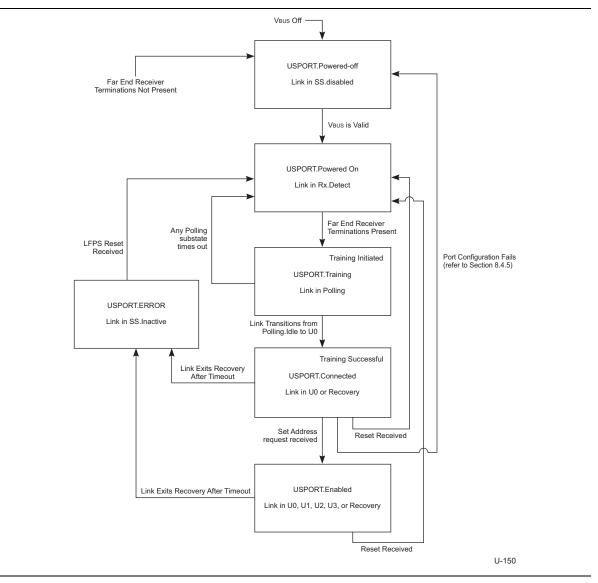
Figure 10-11. Upstream Facing Hub Port State Machine
