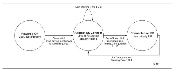
Figure 10-12. Hub Connect State Machine
