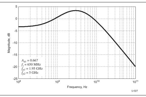
Figure 6-17. Tx Compliance Rx EQ Transfer Function
