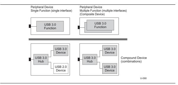
Figure 3-4. Examples of Supported SuperSpeed USB Physical Device Topologies
