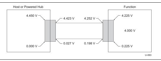
Figure 11-5. Worst-case Voltage Drop Topology (Steady State)
