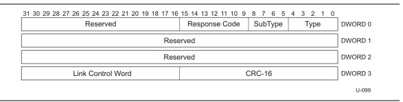
Figure 8-10. Port Configuration Response LMP
