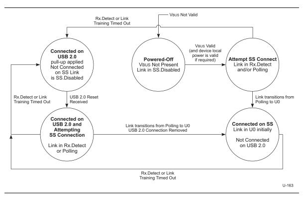
Figure 10-25. Peripheral Device Connect State Machine
