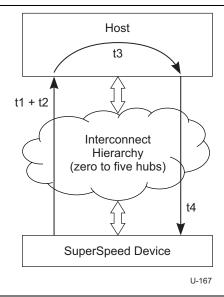
Figure C-2. Device Total Intrinsic Latency Tolerance
