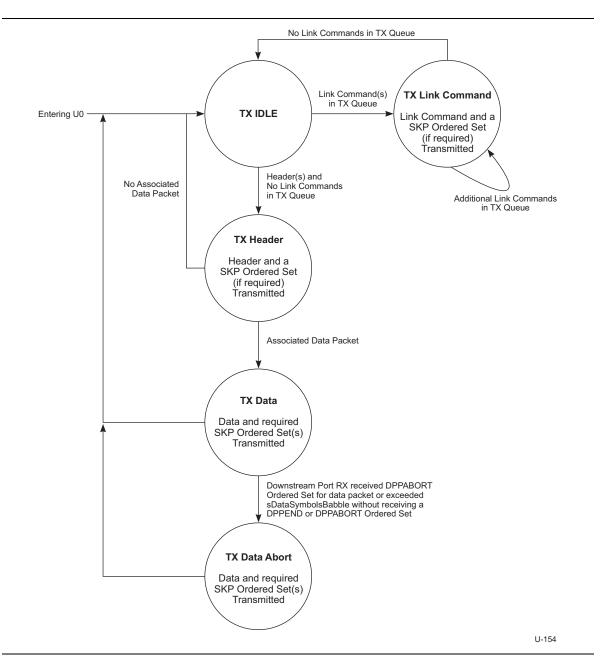
Figure 10-16. Upstream Facing Port Tx State Machine
