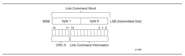
Figure 7-12. Link Command Word Structure
