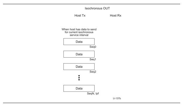
Figure 8-47. Isochronous OUT Transaction Format
