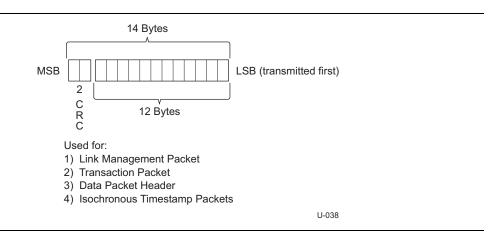
Figure 7-4. Packet Header
