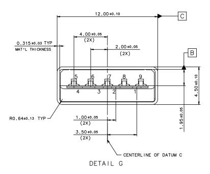
Figure 5-2. USB 3.0 Standard-A Plug Interface Dimensions
