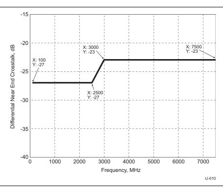
Figure 5-24. Differential Near-End Crosstalk Requirement Between SuperSpeed Pairs
