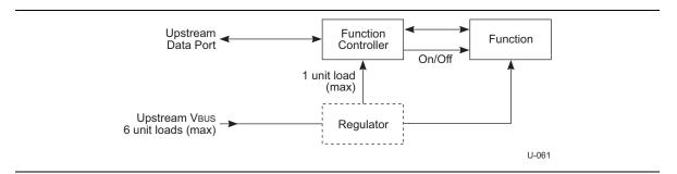
Figure 11-3. High-power Bus-powered Function
