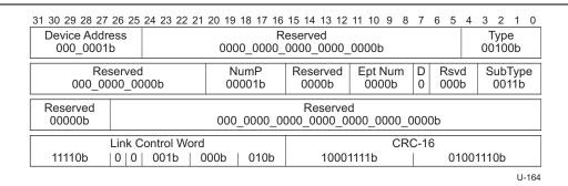
Figure D-1. Sample ERDY Transaction Packet
