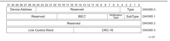
Figure 8-18. Latency Tolerance Message Device Notification
