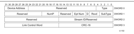
Figure 8-13. ERDY Transaction Packet
