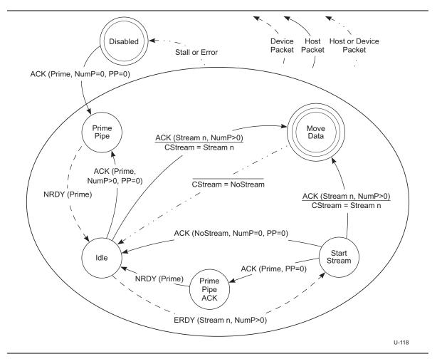
Figure 8-29. Bulk IN Stream Protocol State Machine (ISPSM)
