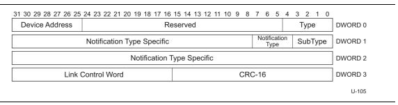
Figure 8-16. Device Notification Transaction Packet
