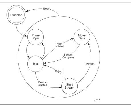
Figure 8-28. General Stream Protocol State Machine (SPSM)
