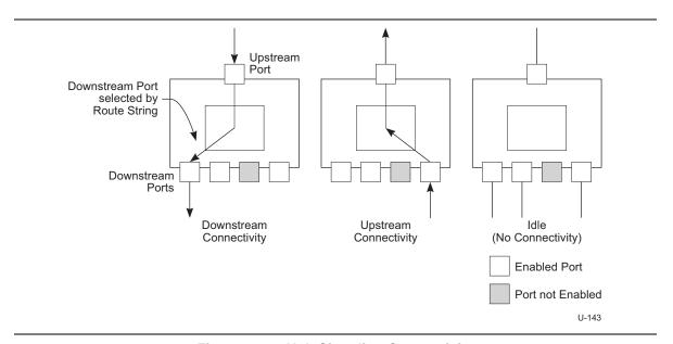
Figure 10-4. Hub Signaling Connectivity
