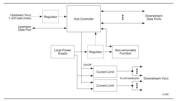
Figure 11-1. Compound Self-powered Hub
