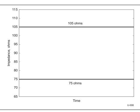
Figure 5-21. Impedance Limits of a Mated Connector
