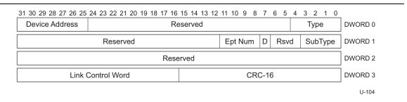
Figure 8-15. STALL Transaction Packet
