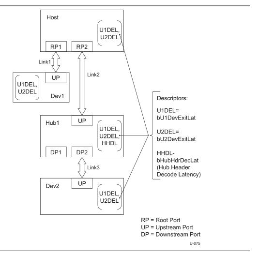
Figure C-3. Host to Device Path Exit Latency Calculation Examples
