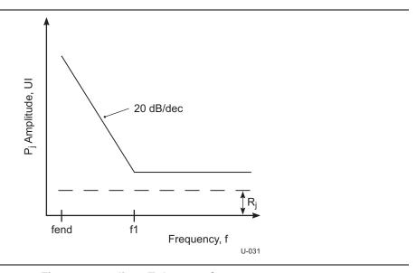
Figure 6-19. Jitter Tolerance Curve
