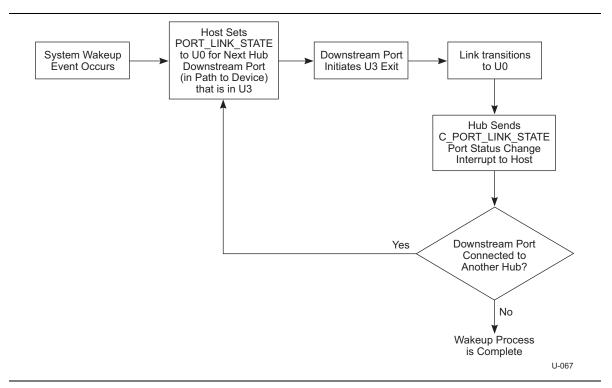
Figure C-1. Flow Diagram for Host Initiated Wakeup
