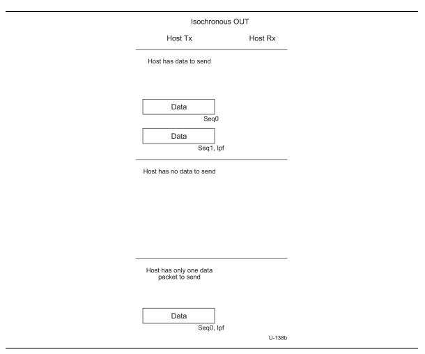
Figure 8-49. Sample Isochronous OUT Transaction
