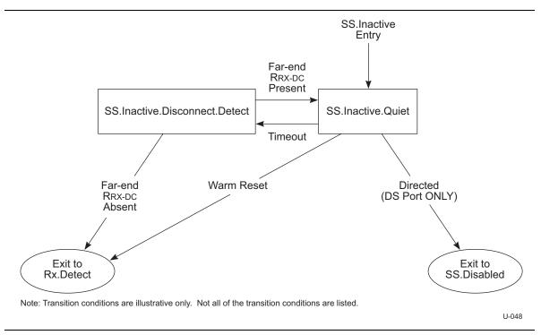
Figure 7-14. SS.Inactive Substate Machine
