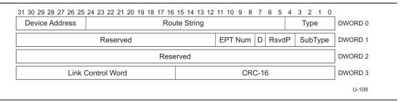
Figure 8-20. PING Transaction Packet
