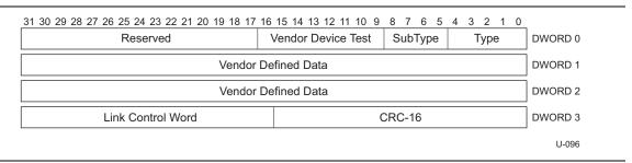
Figure 8-7. Vendor Device Test LMP
