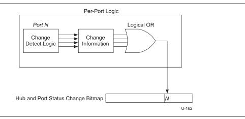
Figure 10-24. Example Hub and Port Change Bit Sampling
