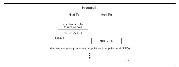
Figure 8-36. Host Stops Servicing Interrupt IN Transaction Once NRDY is Received
