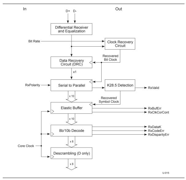
Figure 6-3. Receiver Block Diagram
