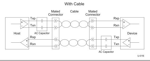
Figure 6-4. Channel Models without a Cable (Top) and with a Cable (Bottom)
