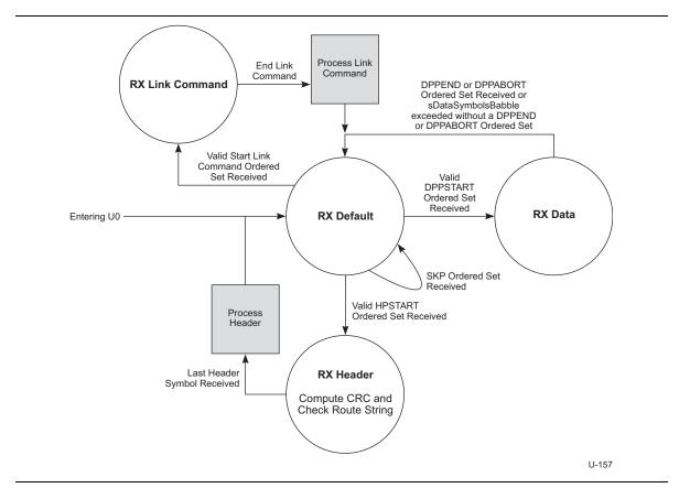
Figure 10-19. Downstream Facing Port Rx State Machine
