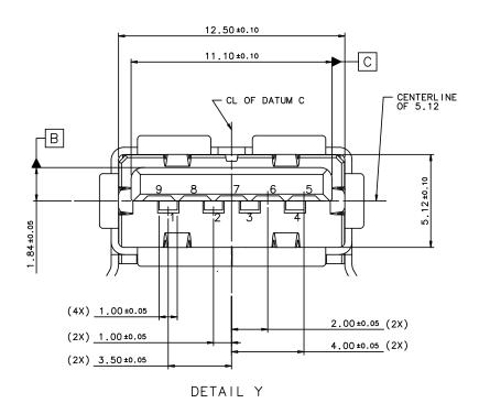
Figure 5-1. USB 3.0 Standard-A Receptacle Interface Dimensions
