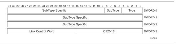
Figure 8-4. Link Management Packet Structure
