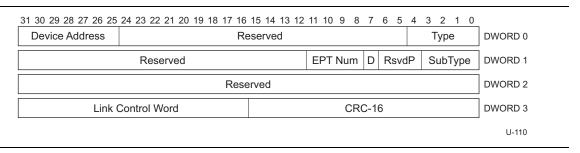
Figure 8-21. PING\_RESPONSE Transaction Packet
