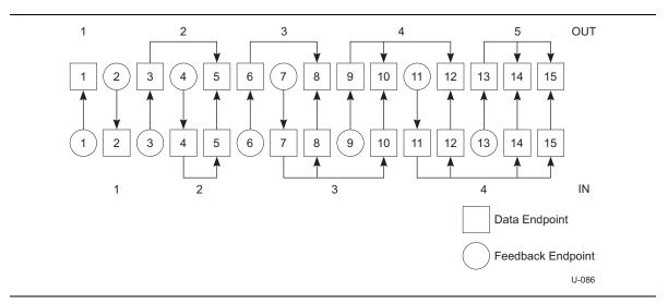
Figure 9-8. Example of Feedback Endpoint Relationships
