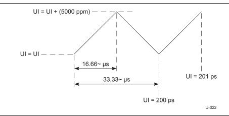
Figure 6-10. Period Modulation from Triangular SSC
