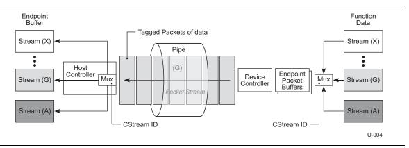
Figure 4-3. USB SuperSpeed IN Stream Example
