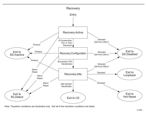
Figure 7-20. Recovery Substate Machine
