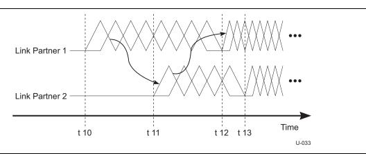
Figure 6-21. U1 Exit, U2 Exit, and U3 Wakeup LFPS Handshake Timing Diagram
