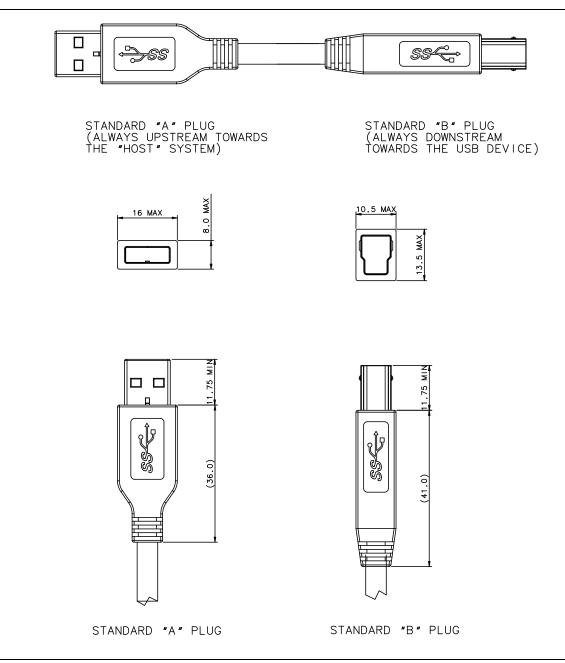
Figure 5-16. USB 3.0 Standard-A to USB 3.0 Standard-B Cable Assembly
