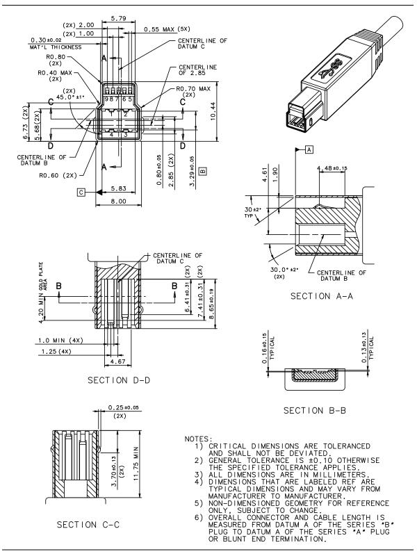
Figure 5-7. USB 3.0 Standard-B Plug Interface Dimensions
