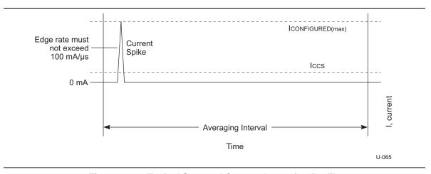
Figure 11-7. Typical Suspend Current Averaging Profile
