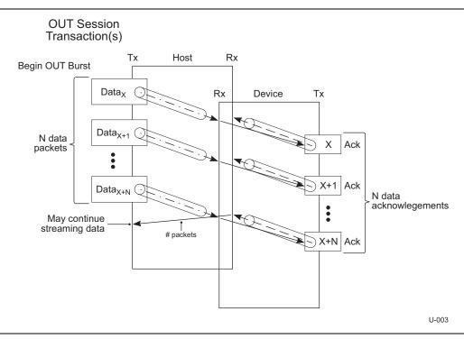
Figure 4-2. SuperSpeed OUT Transaction Protocol
