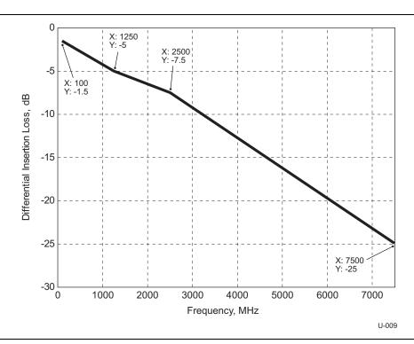
Figure 5-23. Differential Insertion Loss Requirement
