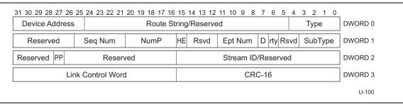
Figure 8-11. ACK Transaction Packet
