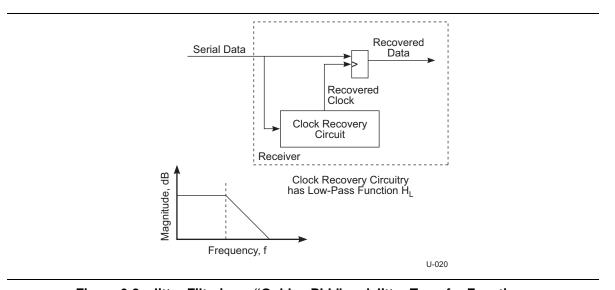
Figure 6-8. Jitter Filtering – "Golden PLL" and Jitter Transfer Functions
