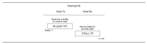
Figure 8-38. Endpoint Sends STALL TP
