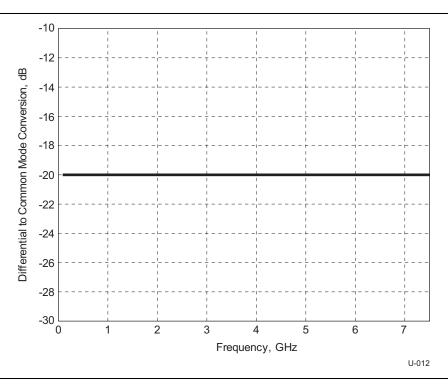
Figure 5-26. Differential-to-Common-Mode Conversion Requirement
