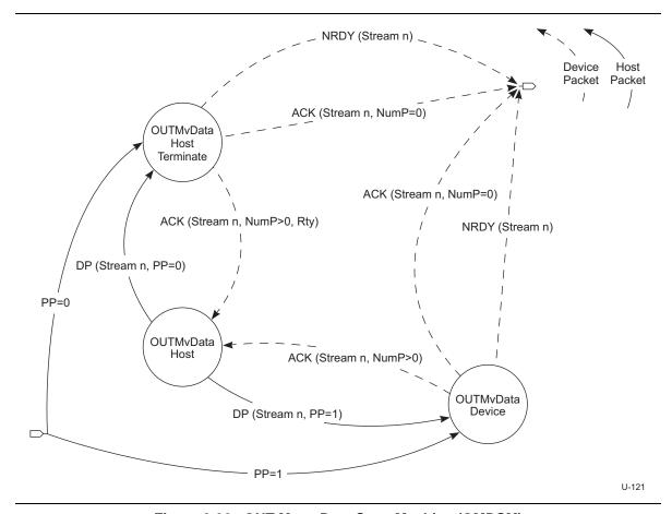
Figure 8-32. OUT Move Data State Machine (OMDSM)
