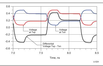
Figure 6-12. Single-ended and Differential Voltage Levels
