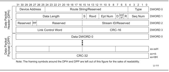
Figure 8-22. Example Data Packet
