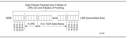
Figure 7-8. Data Packet Payload with CRC-32 and Framing
