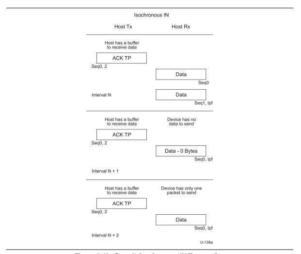
Figure 8-48. Sample Isochronous IN Transaction
