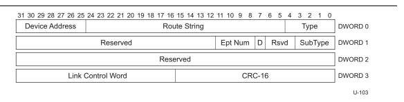
Figure 8-14. STATUS Transaction Packet
