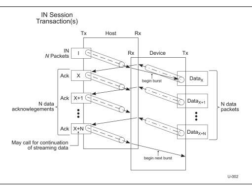
Figure 4-1. SuperSpeed IN Transaction Protocol
