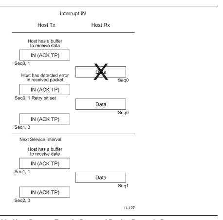
Figure 8-39. Host Detects Error in Data and Device Resends Data
