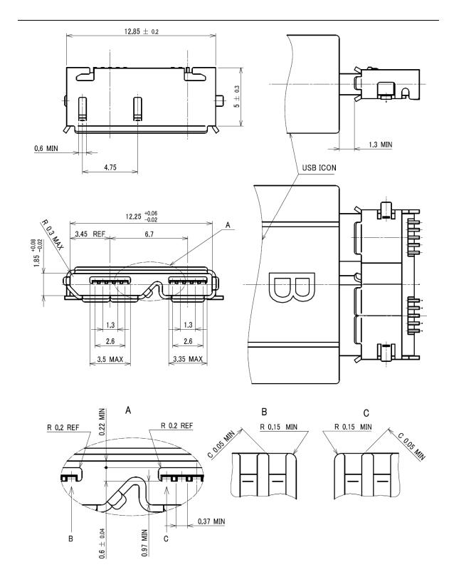
NOTE : General tolerance is  $\pm -0.05$  mm, otherwise the specified tolerances apply.
