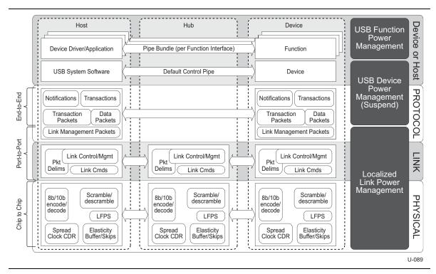
Figure 3-3. SuperSpeed Bus Communications Layers and Power Management Elements
