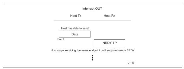
Figure 8-41. Host Stops Servicing Interrupt OUT Transaction Once NRDY is Received
