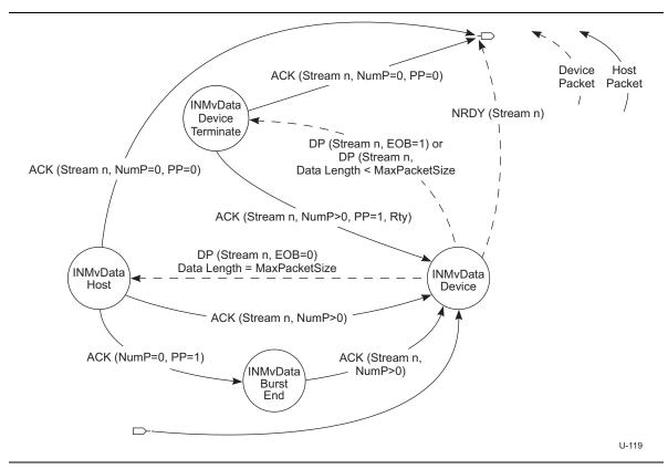
Figure 8-30. IN Move Data State Machine (IMDSM)
