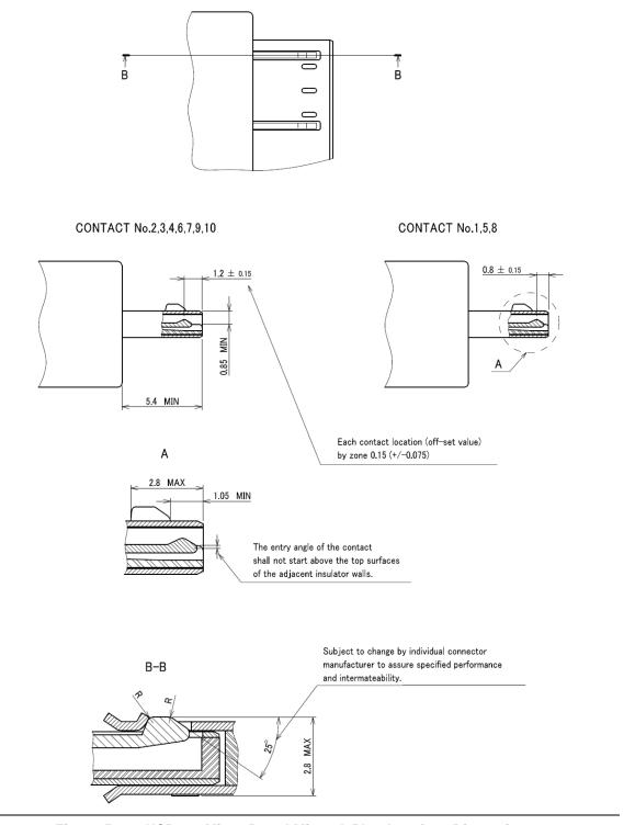
Figure 5-13. USB 3.0 Micro-B and Micro-A Plug Interface Dimensions
