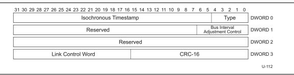
Figure 8-23. Isochronous Timestamp Packet
