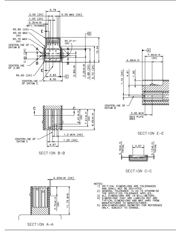
Figure 5-10. USB 3.0 Powered-B Plug Interface Dimensions
