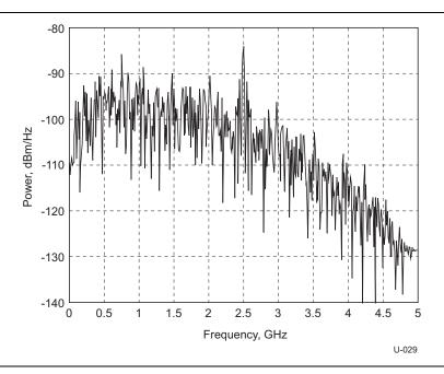
Figure 6-16. Frequency Spectrum of TSEQ
