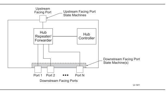
Figure 10-2. SuperSpeed Portion of the Hub Architecture
