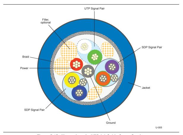
Figure 5-15. Illustration of a USB 3.0 Cable Cross-Section
