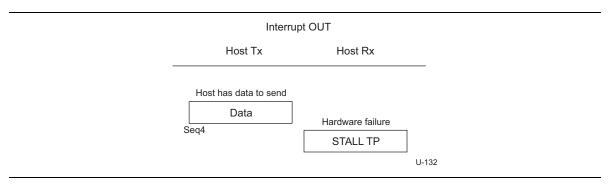
Figure 8-44. Endpoint Sends STALL TP
