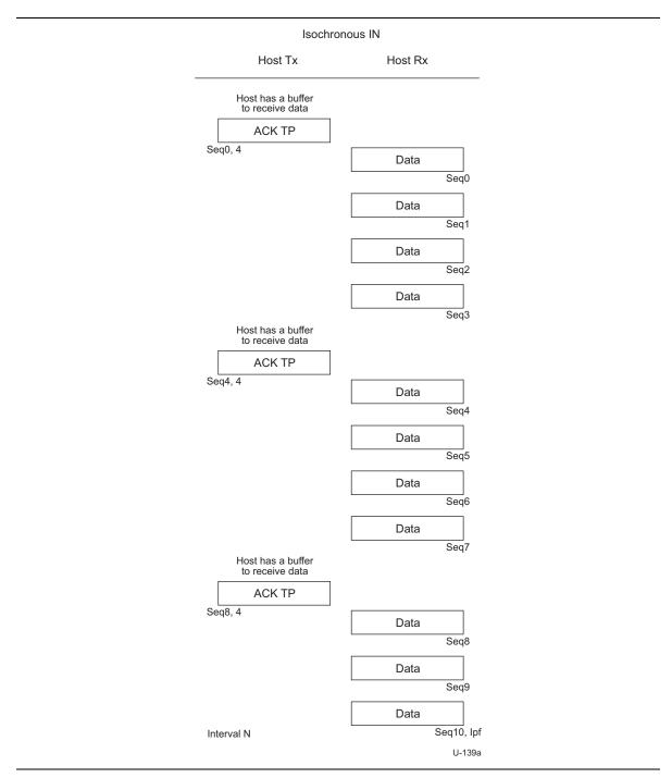
Figure 8-50. Isochronous IN Transaction Example
