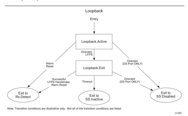
Figure 7-21. Loopback Substate Machine
