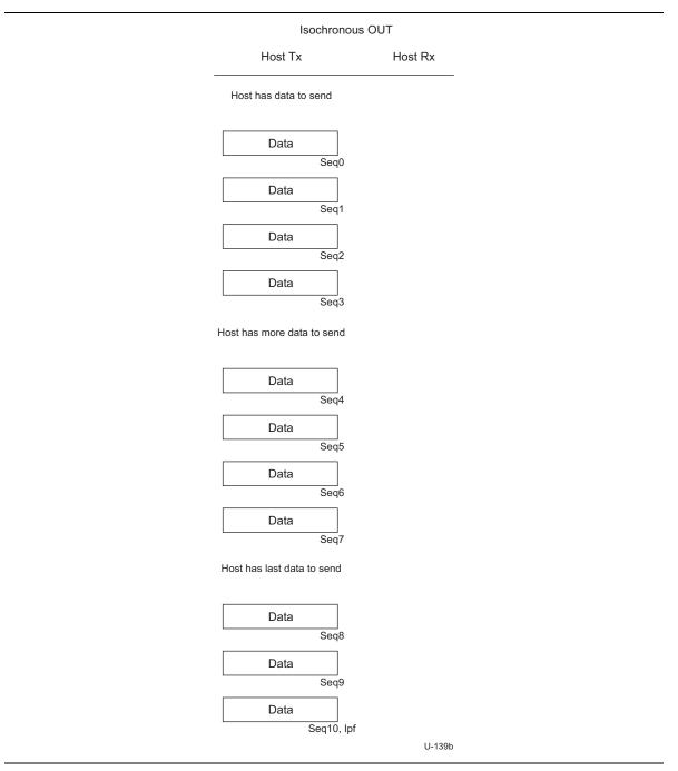
Figure 8-51. Isochronous OUT Transaction Example
