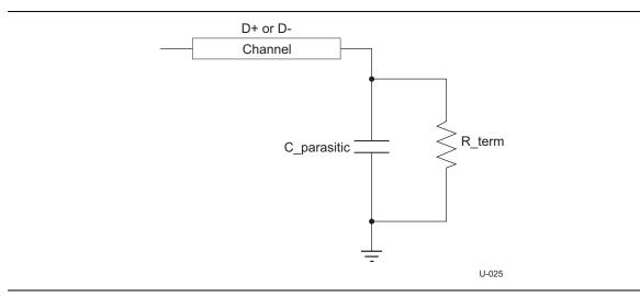
Figure 6-13. Device Termination Schematic
