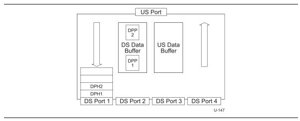
Figure 10-8. Hub Data Buffer Traffic (Header Packet Buffer Only Shown for DS Port 1)
