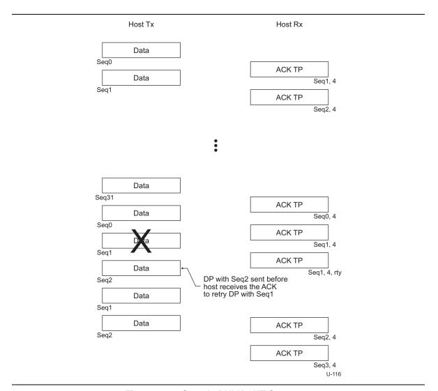
Figure 8-27. Sample BULK OUT Sequence
