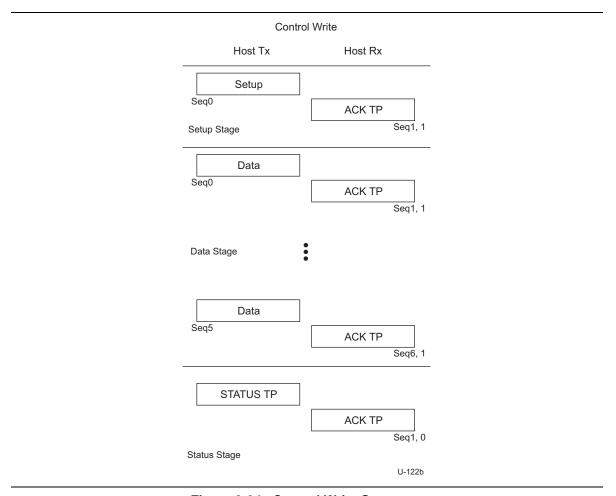
Figure 8-34. Control Write Sequence
