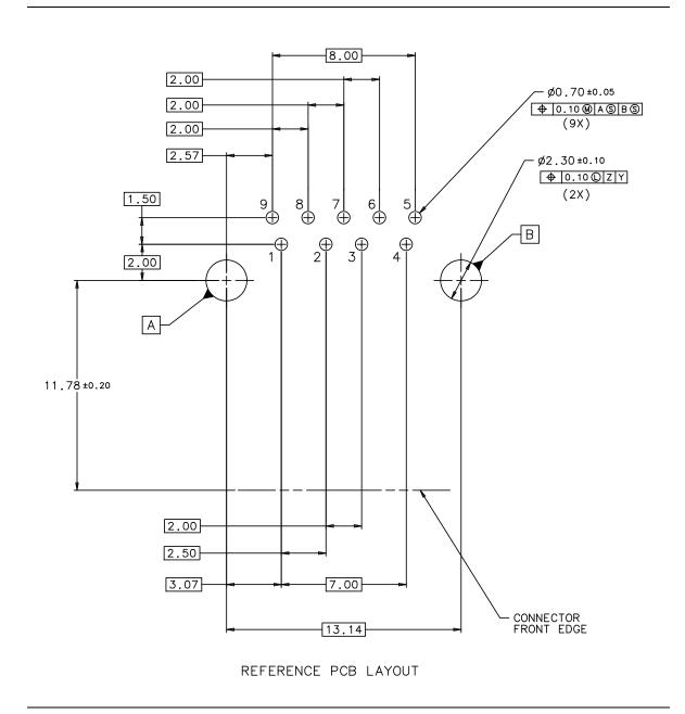
Figure 5-3. Reference Footprint for the USB 3.0 Standard-A Receptacle
