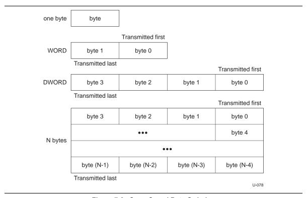
Figure 7-2. SuperSpeed Byte Ordering
