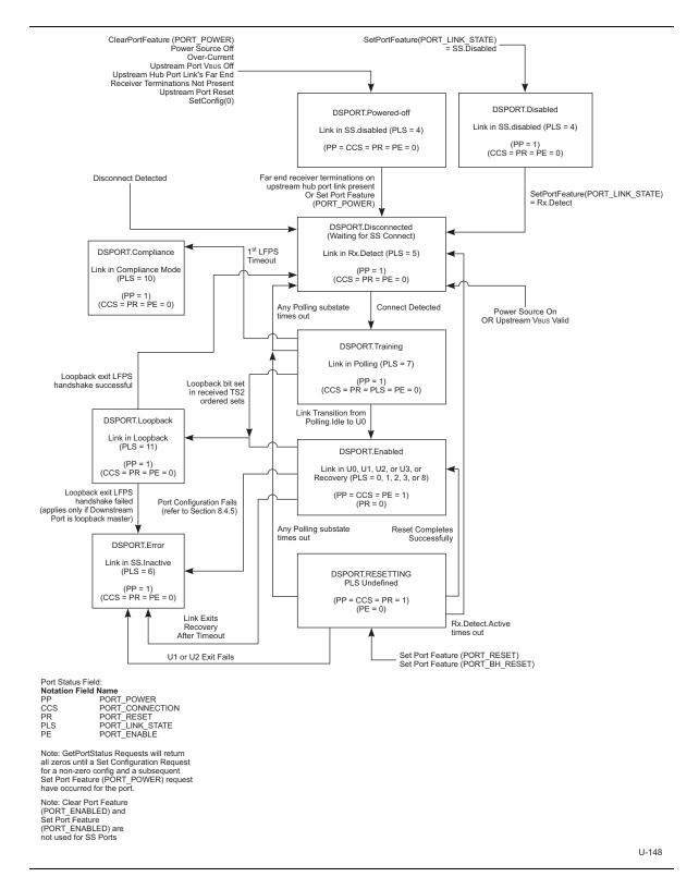
Figure 10-9. Downstream Facing Hub Port State Machine
