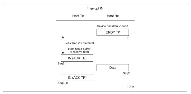
Figure 8-37. Host Resumes IN Transaction after Device Sent ERDY
