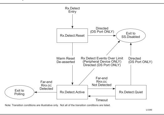
Figure 7-15. Rx.Detect Substate Machine
