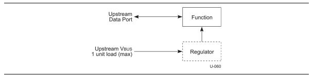
Figure 11-2. Low-power Bus-powered Function
