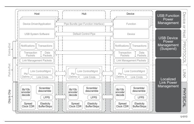
Figure 6-1. SuperSpeed Physical Layer
