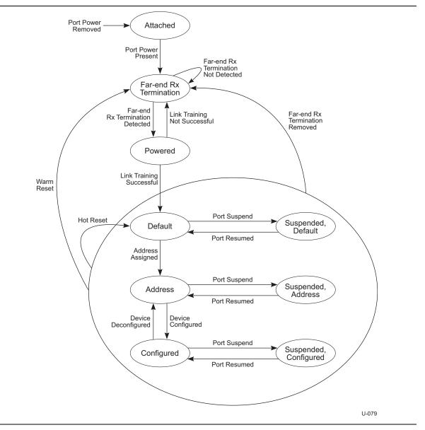
Figure 9-2. Hub State Diagram (SuperSpeed Portion Only)
