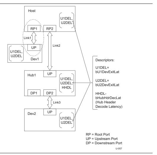
Figure C-4. Device Connected Directly to a Host
