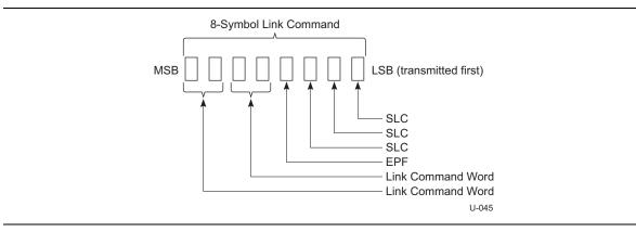
Figure 7-11. Link Command Structure
