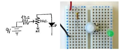
Lastly, the LED's cathode is connected to the negative terminal of the battery to complete the circuit.
