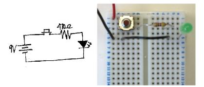
And you've successfully wired your second circuit! Just connect your battery and verify that when you press the button, the LED lights up.
