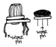
Potentiometers come in all sorts of shapes and sizes, but their functionality remains the same across most types. They have three pins, two of which make up the total resistor value, and a third called the wiper. The wiper is the actual mechanism that changes the resistance value as you rotate the dial. This is normally the center pin on most potentiometers, and an example drawing of two commonly found potentiometers can be seen to the left.
