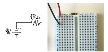
Then, the other end of the resistor is connected to the anode (or long lead) of the LED:
