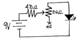
The potentiometer is also known as a variable resistor which, as its name implies, has a resistance that changes. The  $10k\Omega$  marking next to the schematic symbol indicates the maximum resistance value the potentiometer has.
