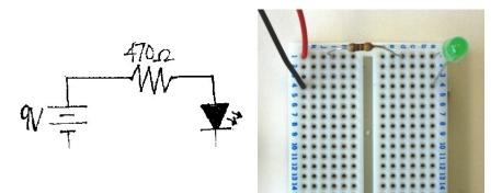
Finally, the cathode of the LED is connected to the negative terminal of the battery, like so:
