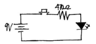
The pushbutton is interesting in that it has four pins, but is only represented in a schematic by two. This is because the pushbutton needs all four pins for stability, but only two for functionality. The two pins not shown in the schematic symbol are electrically connected to the two pins that are shown and therefore not necessary to picture.
