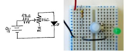
Now, when you plug the battery into the clip, the LED should become brighter or dimmer depending on the direction of rotation.
