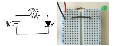
And congratulations, you've successfully wired a circuit from a schematic! That wasn't so horrible, was it? Now if you plug a battery into the clip, the LED should light up.
