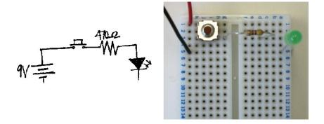
And finally, the cathode of the LED is connected to the negative terminal of the battery:
