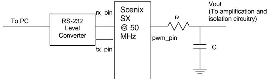
To calculate the component values for a cutoff frequency of 1633 Hz, first the value of R must be chosen.
