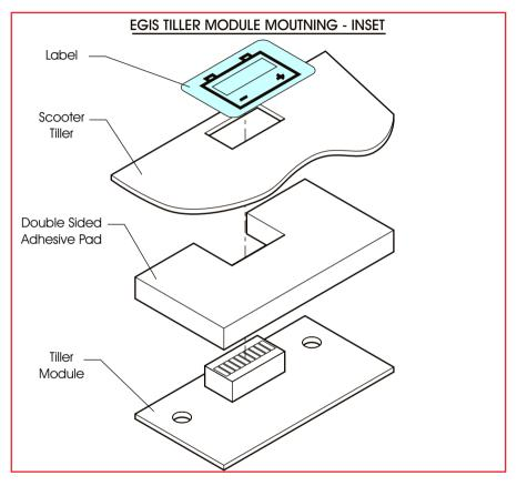
The module should be sealed against the ingress of water and dust by a placing an adhesive waterproof overlay over the display cut-out. The overlay should contain a suitably sized transparent window and the overall dimensions should be at least 36.0mm x 20.5mm (1.41" x 0.81")
