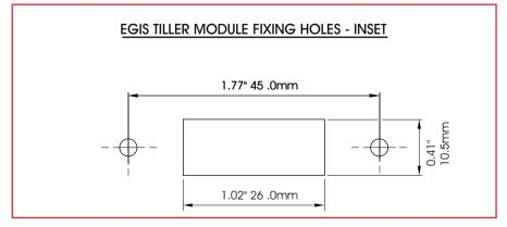
Alternatively M3 (4-40 UNC) hardware can be used. The height of the display from the printed circuit board is 8.0mm (0.31"). Suitable spacers should be used so that the display is fixed slightly below the scooter's control panel. Ensure that the metallic fixing hardware (nuts, washers etc.) do not touch the conductive tracks on the printed circuit board.
