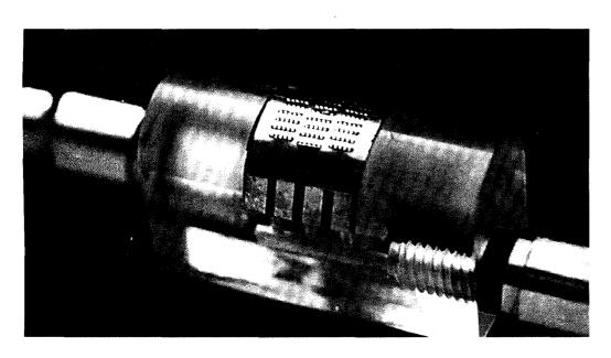
Micro size fuel cell made from polymeric and metal foil supplies 160 mW from 1 cm<sup>2</sup>.
